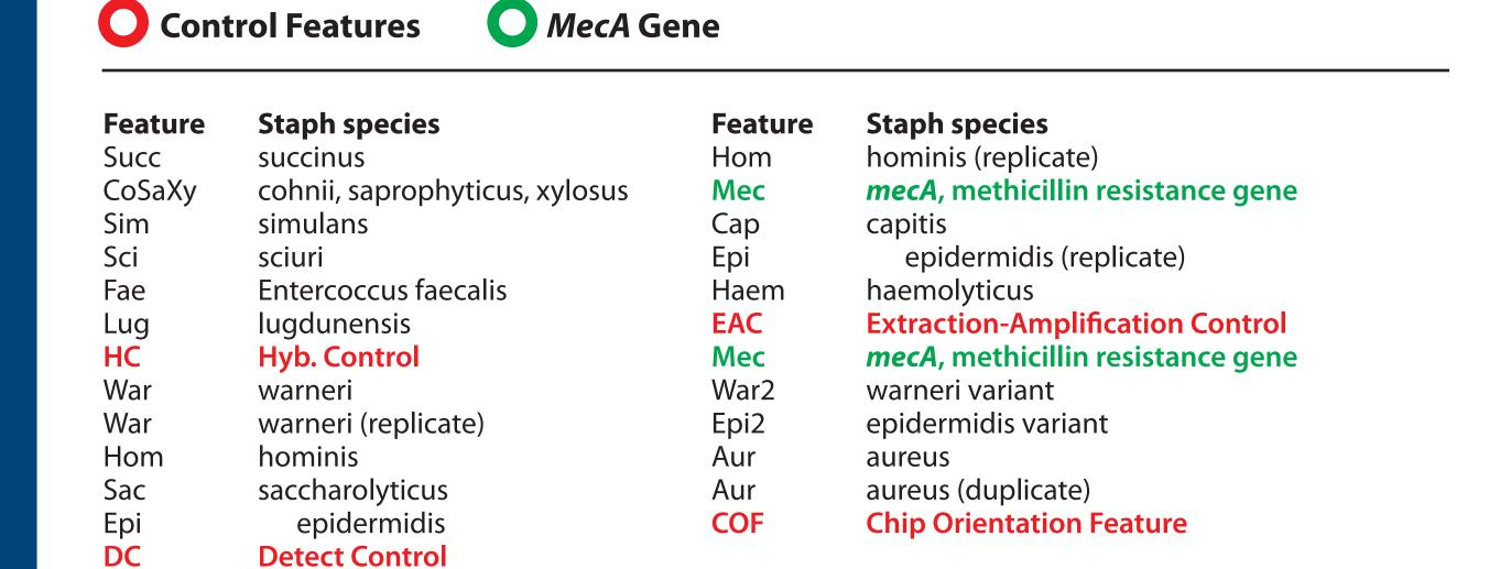
Capture probes are immobilized to the silicon surface. A diagonal set of control features verifies that chip orientation (COF), DNA extraction and amplification (EAC), and **detection** (HC, DC) functioned properly, validating test results.
