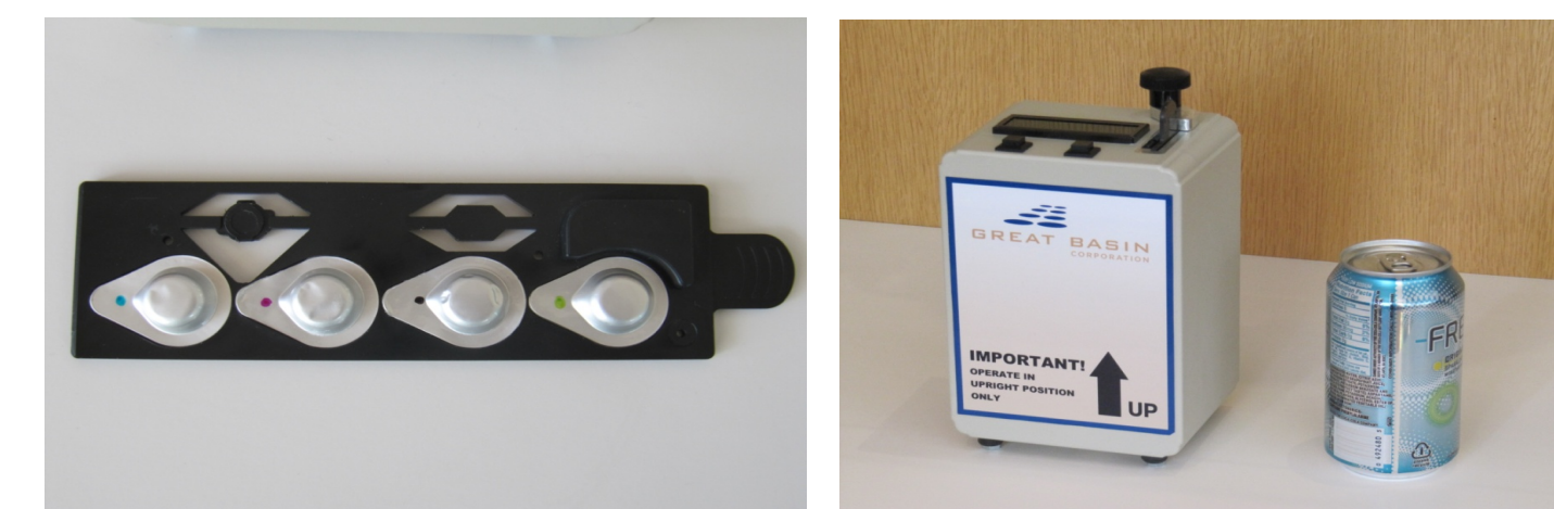
Figure 6. TB ID/R Assay Automation. The assay is currently being automated on a cartridge-based compact device. (Left) A cartridge is shown with four blisters packaged with four different assay reagents at the bottom row and the amplification and detection chambers on the top row. (Right) A prototype device is shown with the cartridge loaded on the top right side (a soft drink aluminum can was photographed for easy comparison of the device dimensions).
